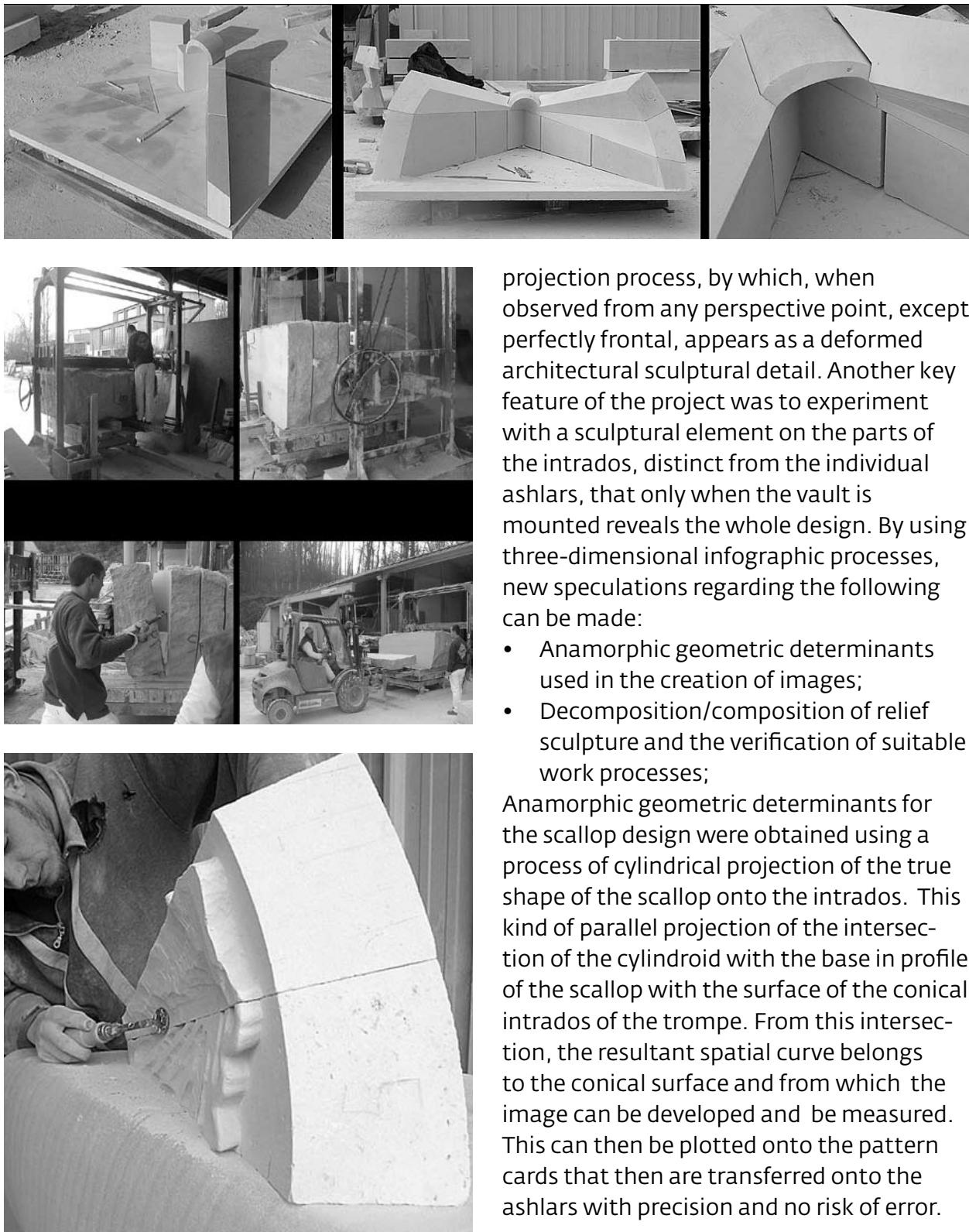
projection process, by which, when observed from any perspective point, except perfectly frontal, appears as a deformed architectural sculptural detail. Another key feature of the project was to experiment with a sculptural element on the parts of the intrados, distinct from the individual ashlar, that only when the vault is mounted reveals the whole design. By using three-dimensional infographic processes, new speculations regarding the following can be made:
