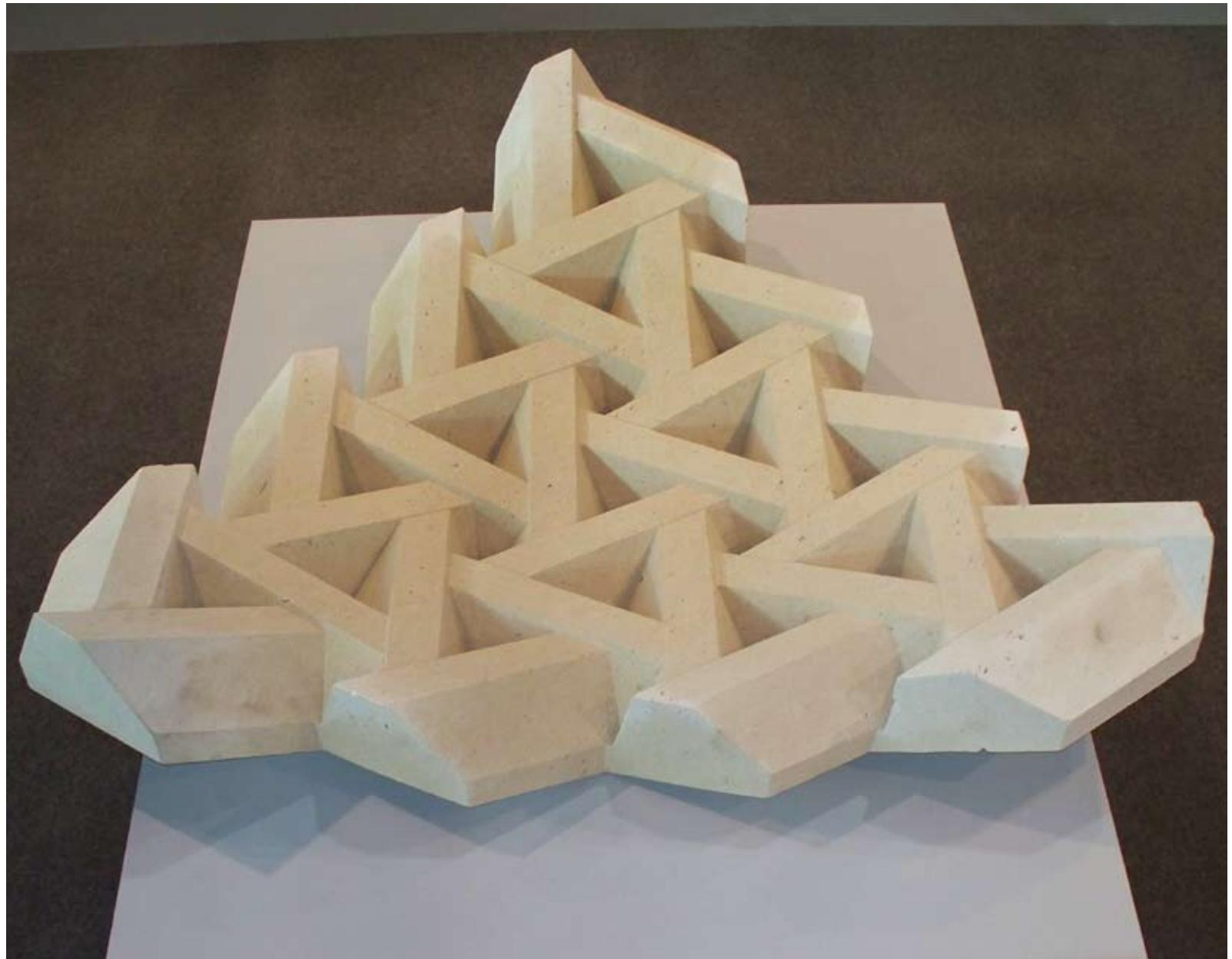
This prototype investigates the geometrical problems connected to the tiling of surfaces and is a concrete solution to the contemporary demands of the building industry to remain competitive and cheap in the construction of spherical vaults with plaited intrados.
