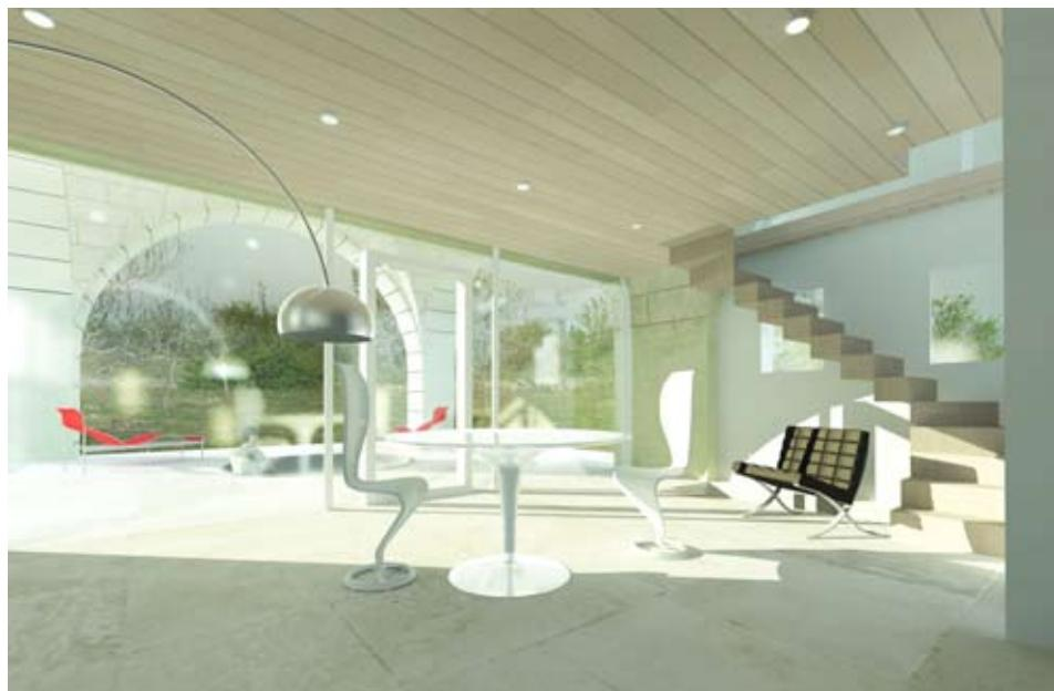
The walls are made of stone (Apricena and Trani limestone for the vertical systems, tufa from Canosa or Gravina for the square vaults) cut thickly to ensure that the stone mass, in association with the underground area beneath the house, can regulate the temperature inside the house in the Summer. The external façade of the house has a mixture of opaque stone facings and transparent glass, to allow for a view. The stone façade is made of local stone and white lime plaster.
